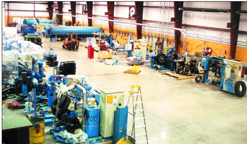
The rebuilding area features air and electric hook-ups that allow testing of all new and used equipment – before shipment to the customer and during the rebuilding phase.
