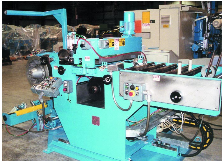
After rebuilding, this precure builder is ready for shipment.
