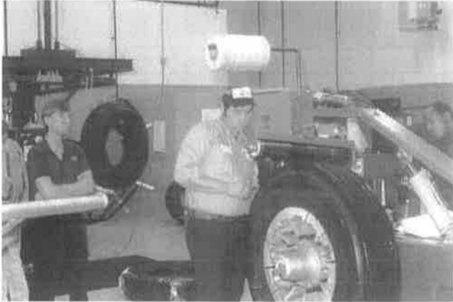
This is a classic example of a student "eye-balling" the tread to see if it is centered and straight on the truck tire casing during the precure building process at the training center.
