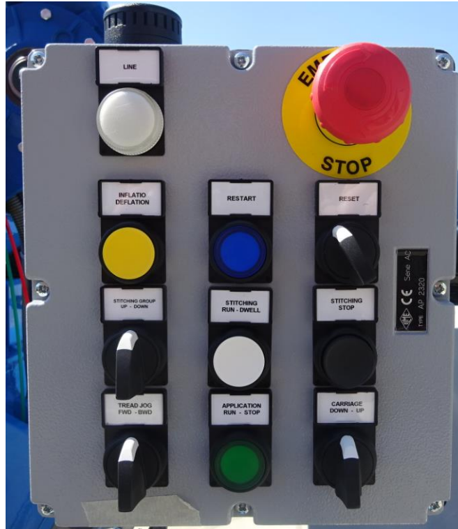
Figure 12: building zone control panel
