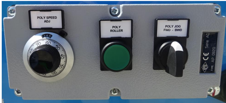
Figure 14: poly zone control panel
